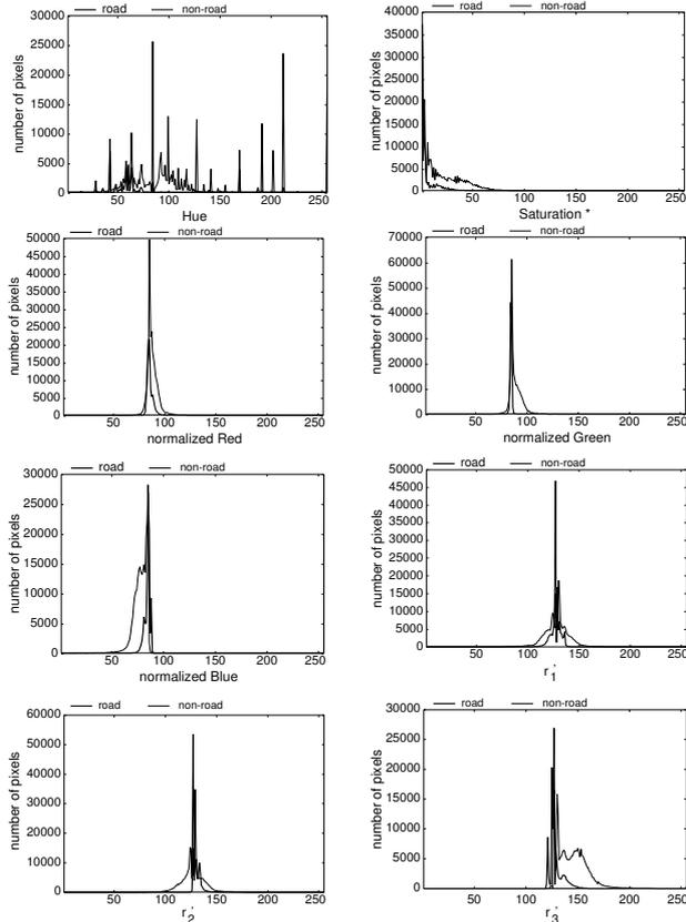
Figure 6: Histogram analysis of the road scene in Fig. 5.  $r_3$  has the highest value of  $\kappa$  calculated by Eq.(17).
