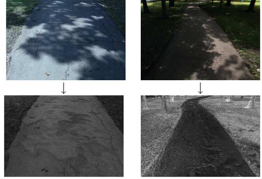
Figure 4: Results of feature selection for road segmentation in different test roads. Upper images are input and lower images are the output of selected color channel with highest value of  $\kappa$  calculated by Eq.(17).
