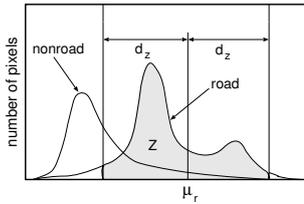
Figure 3: The definition of zone  $z$  in of road and non-road histogram. For a given  $z$ , the feature  $f$  is evaluated by Eq.(17).
