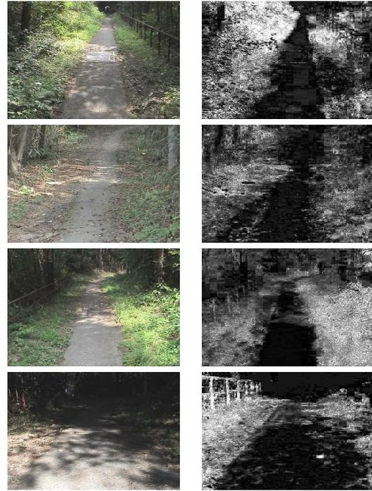
Figure 7: Results of color selection for road segmentation in our test field. Darker regions have similar values to the road color.
