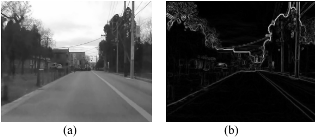
Figure 2: (a) Input image. (b) Result of edge detection.
