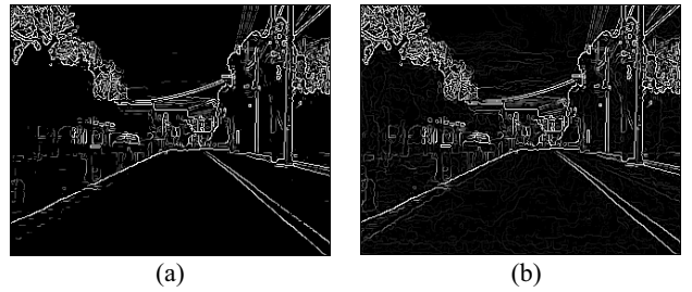
Figure 3: Thinning and binarization (a) the threshold value by the discriminant analysis method. (b) the fixed threshold.
