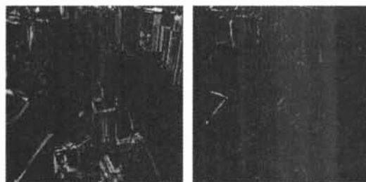
Figure 5: Difference images for time steps 4 and 7 of the Rotor sequence from similar camera positions before and after refinement.
