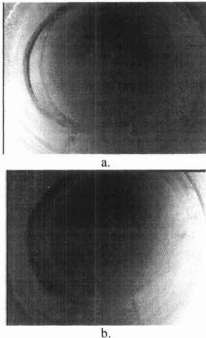
Figure 1. A lateral junction viewed under a) direct and b) reflected illumination. Images were acquired using a Watec CCD camera mounted on a sewer-going tractor [2] and a DT Fidelity 100 frame grabber.
