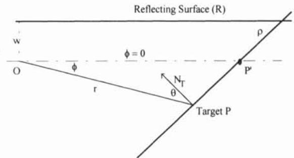
Figure 2: The geometry of direct illumination
