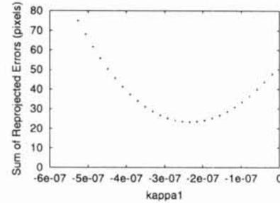
Figure 4: Error curve by varying the radial distortion coefficient  $k$
