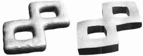
Fig. 5: Left: a polygonal two-holed torus. Right: the ridges are sharpened after adaptive smoothing and provide with a natural decomposition of the two-holed torus.
