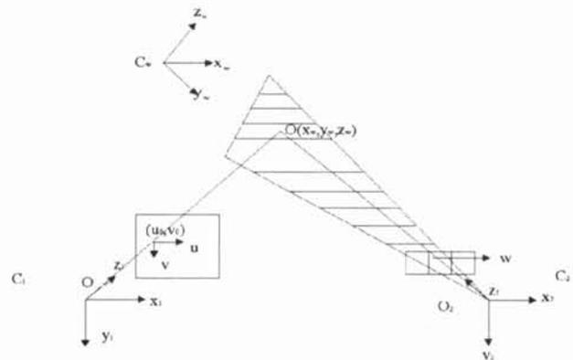
Figure 1: Determination of depth from a structured light.
