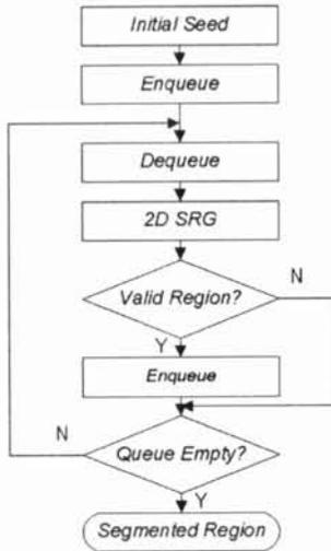
Figure 4: Algorithm of the Slice-based 3D SRG
