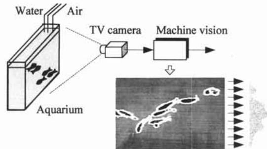
Fig. 16 Water purity monitoring from fish behavior (1990)
