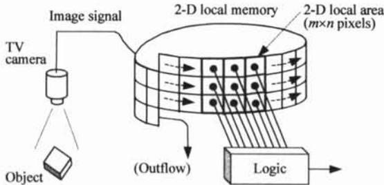
Fig. 4 Local-parallel processing hardware
