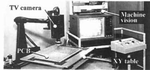
Fig. 6 Inspection of PCBs and its principle (1972)
