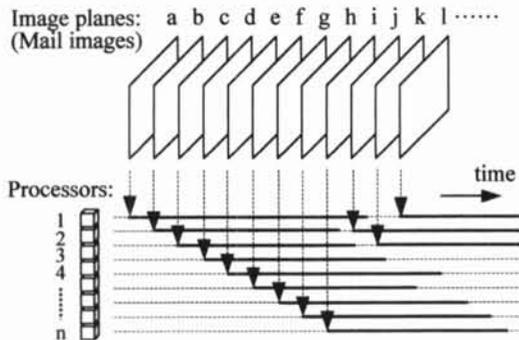
Fig. 13 Temporarily-parallel processing by multi-microprocessors
