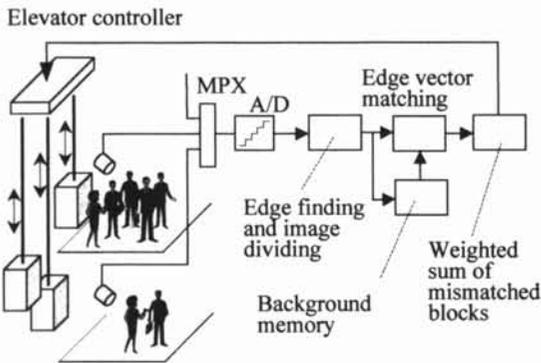
Fig. 15 Elevator eye system (1977)
