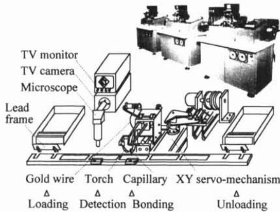
Fig. 8 Transistor assembly machine (1973)
