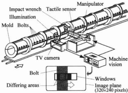
Fig. 5 Bolting robot for concrete piles/poles (1972)
