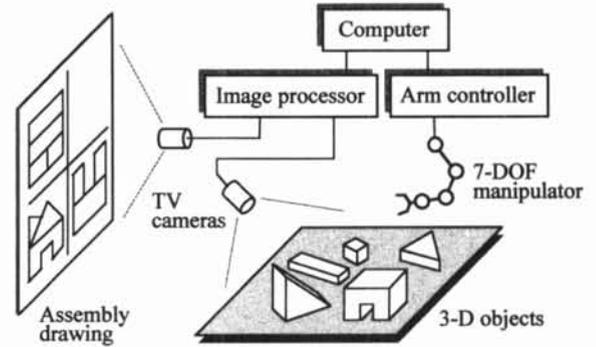
Fig. 3 Intelligent assembly robot (1970)
