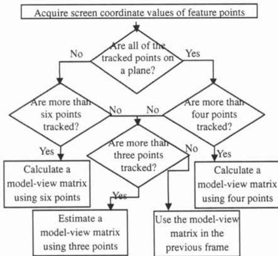
Figure 5 : A process of model-view matrix calculation.
