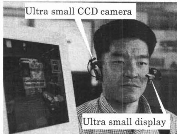
Figure 1: Appearance of a user of the system
