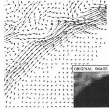
Figure 1. : Rotation vector representation of welded surface image around crack
