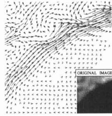
Figure 1. : Rotation vector representation of welded surface image around crack
