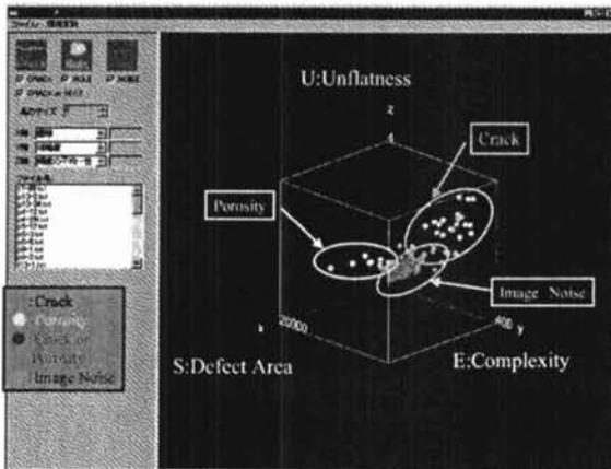
Figure 5. : Feature space plot for the defect type identification
