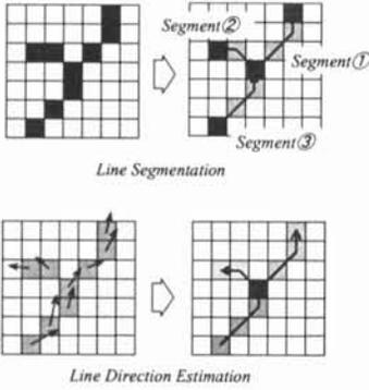
Figure 3. : Illustration of line segmentation and direction estimation process
