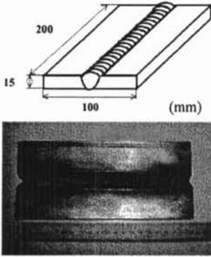
Figure 4. : Appearance and size of test piece
