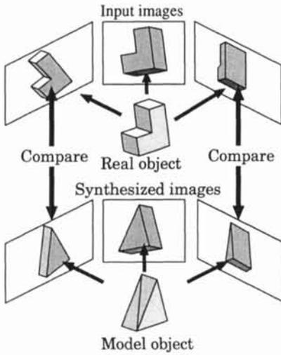
Figure 1: Concept for the proposed 3-D shape reconstruction method
