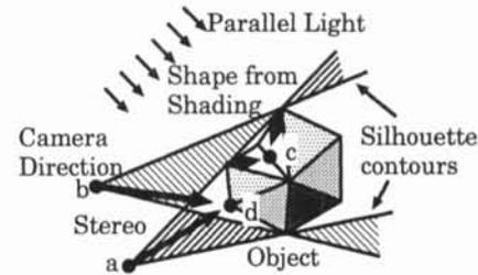
Figure 13: Fusion of stereo, silhouette contours, and shape from shading
