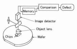
Fig. 2 Inspection principle
