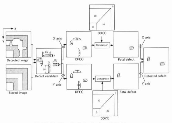
Fig. 3 Principle of Geometrical Feature-Based Image Comparison
