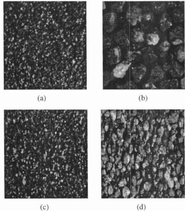
Figure 3. a) grain fraction  $37\ \mu\text{m}$ - $44\ \mu\text{m}$  b)  $420\ \mu\text{m}$ - $500\ \mu\text{m}$  c) mixture of fractions  $37\ \mu\text{m}$ - $44\ \mu\text{m}$ ,  $44\ \mu\text{m}$ - $53\ \mu\text{m}$  and  $53\ \mu\text{m}$ - $62\ \mu\text{m}$  d) mixture of fractions  $149\ \mu\text{m}$ - $177\ \mu\text{m}$ ,  $177\ \mu\text{m}$ - $210\ \mu\text{m}$  and  $210\ \mu\text{m}$ - $250\ \mu\text{m}$
