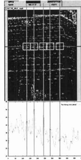
Figure 3: Clustering peaks based on the distribution of the points locating in the particular windows
