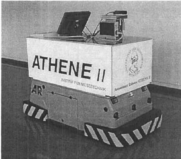
Figure 5: ATHENE II, a vision-guided mobile robot.
