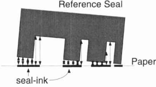
Figure 3: Definition of the normalized range . (Arrows show the range.)
