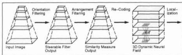
Figure 3: Processing steps for person localization. Starting from a multi-resolution representation of the image, each level is treated by steerable filters. Applying the filter arrangement we determine a distance measure which is taken as input of a three-dimensional field of dynamic neurons. The resulting blob (locally delimited pattern of active neurons) is used to localize a person.
