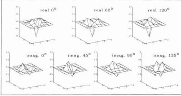
Figure 2: The basis filter set: upper row with 3 basis functions (second order derivative of Gaussian), bottom row with 4 more basis functions (Hilbert transform of the second derivative of Gaussian).
