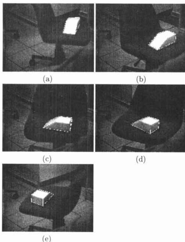
Figure 3: Snap shots of the real time tracking. The wedge model is predefined in the database and the tracking is performed based on the projection of the model matching against the sensed image with defined control points.
