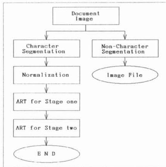
Figure 2. The overview of ART based neural network hierarchy
