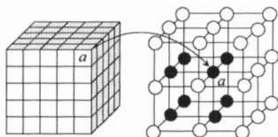
**Figure 2.** Point  $a$  in a cube of  $5 \times 5 \times 5$  voxels and its 26-neighbors. Point  $a$  is said to be deletable by the template  $T_1$  in Figure 1. The 26-neighbors of point  $a$  match template  $T_1$ .
