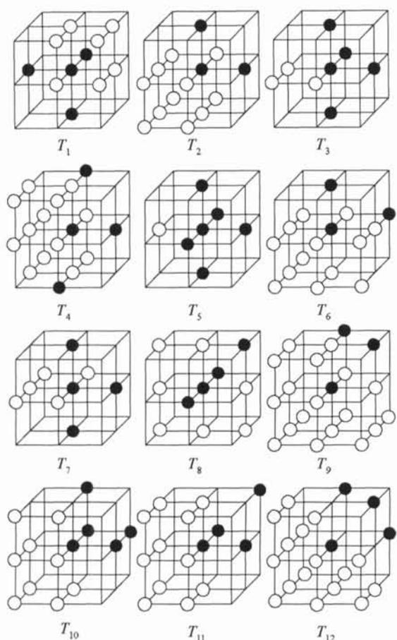
**Figure 1.** Examples of templates for the three-dimensional thinning. The solid circles are black points which are 26-connected to each other and the open circles are white points which are 6-connected to each other. Deletion of the center voxel (black point) does not change the connectivities of either the black or white points.
