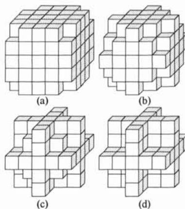
**Figure 4.** Intermediate figures (a), (b) and (c) in the thinning process using the set of templates  $\{T_1\}$ . No further changes occur in the following process. This is the converged result (d).
