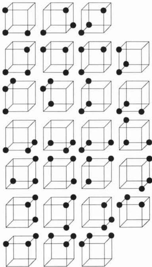
Figure 5. Three fundamental patterns (top three) to check of one-voxel-thickness. They are independent of each other. Each of them has twenty-three symmetrically rotated patterns. Symmetrically rotated patterns of the first fundamental pattern are shown from the second row. All seventy-two patterns are used for this purpose.
