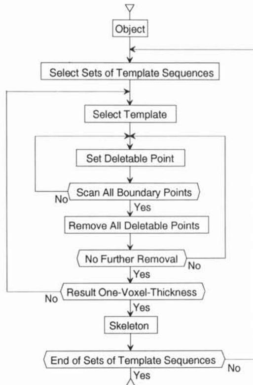
Figure 6. Flow chart of the thinning process for multiple skeletons. We prepared twelve sets of templates and seventy-two one voxel checking patterns.
