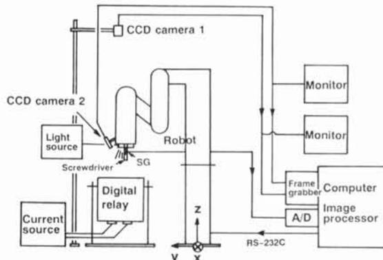
Fig.1 Schematic diagram of RDS switching system. SG:strain gauge
