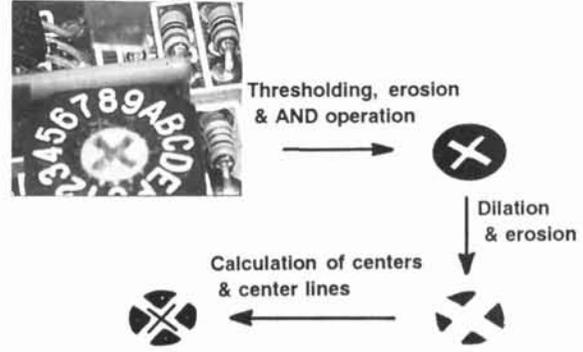
Fig.5 Algorithm for determining RDS groove position in an image.
