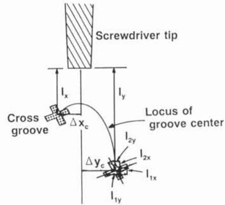
Fig.6 Position change of cross groove image in a scene by rotation of robot-hand head.  $l_{1x}$ ,  $l_{1y}$ ,  $l_{2x}$  and  $l_{2y}$  are x and y components of the center line in each groove, respectively. (Cross groove before and after rotation are indicated by hatching and dots, respectively. Position of screwdriver in the scene does not change.)
