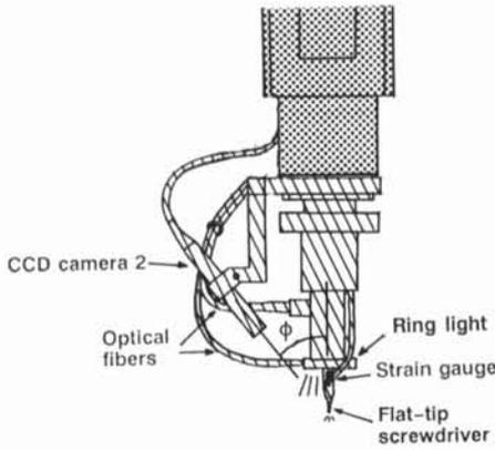
Fig.2 Expanded view of robot hand head.
