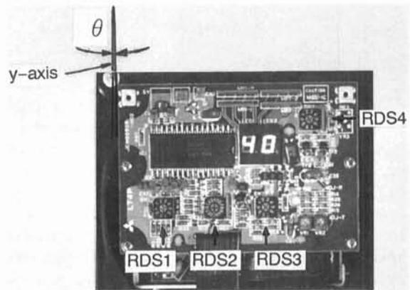
Fig.3 A relay board image observed with CCD camera 1.
