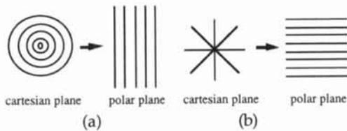
Figure 4 The polar mapping results in the transformation of certain regular patterns in the z-plane into other regular patterns in the w-plane.
