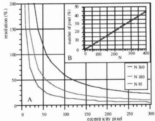
Fig6. (A). Percent variation of resolution as a function of eccentricity for different values of image line N. (B) Percentage of the number of elements a given field as a function of N.
