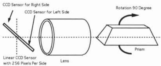
Fig.7 Construction of the image rotation system
