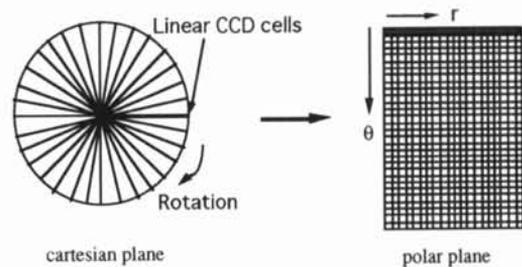
Figure 5 Method of increasing sensor density towards the center of the visual field
