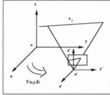
Figure 1: The world and robot co-ordinate systems
