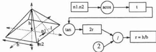
Figure 1: Pyramid example: (a) a pyramid with observations  $n_1$  and  $n_2$  on a side and on the base respectively; (b) network connections for propagation of image-measurements to model parameters. The squares represent variable nodes, the circles represent operation and constant nodes.
