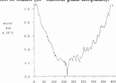
Fig (i) The merit function for a fine X-search scan along the "right" row. Note 16 pixel "dip" width.
