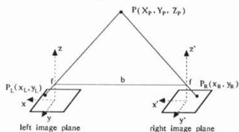
Fig. 2 The lateral stereo camera model.
