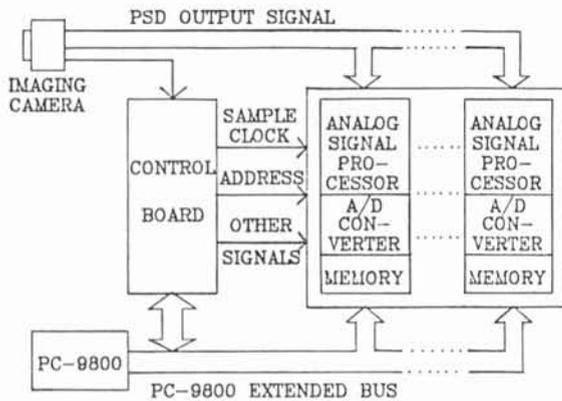
Fig.4 Block diagram of configuration of trial system.
