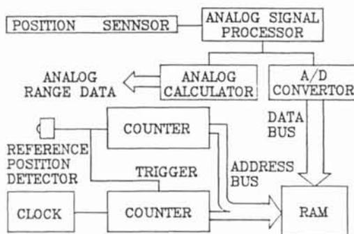
Fig.3 Block diagram of signal processing part.
