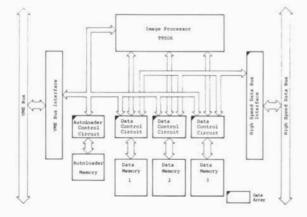
Fig. 3 Fundamental Schematic Diagram of VME Processor Board
