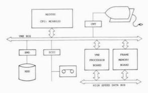
Fig. 7 Example of EWS Image Processor System
