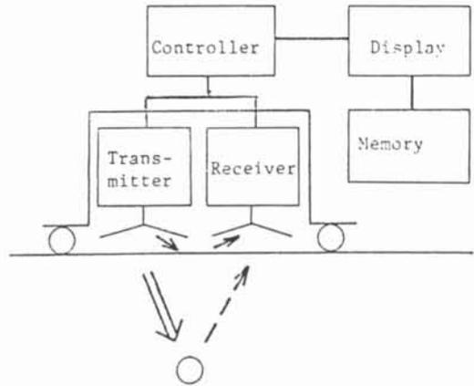
Fig.5 System configuration
