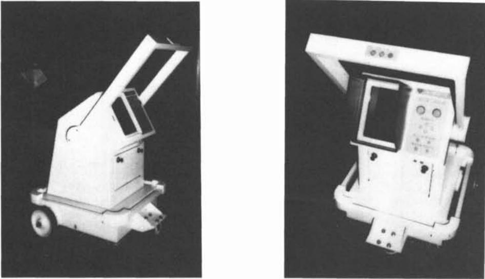
Fig.6 Compact underground radar system
