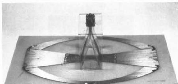
Fig.1 Three-dimensional tower-shaped antenna
