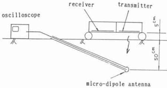
Fig.2 Measurement system
