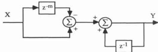
Figure 1. Block diagram of the mean filter.
