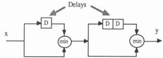
Figure 4. Block diagram of the minimum filter on a set of 4 samples.
