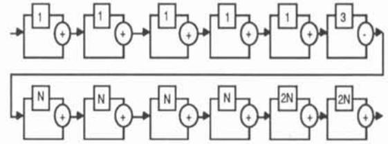
Figure 3. Block diagram of the 9x9 east edge extractor.
