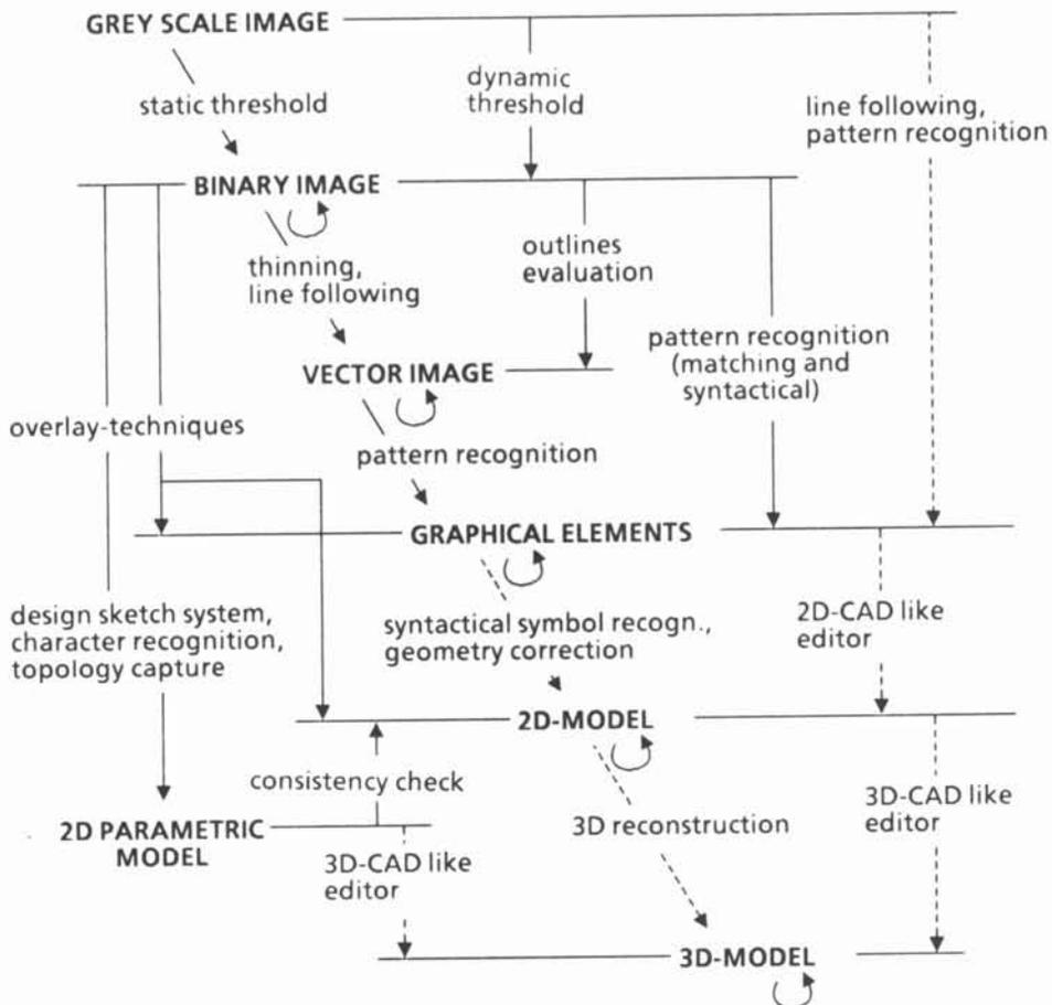
Fig. 1: Schema of drawing conversion processes
