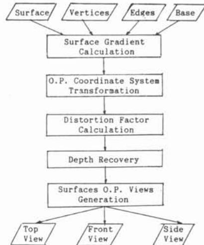
Figure 4. O.P. Views Generation Flow Diagram.
