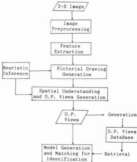
Figure 2. System Configuration.
