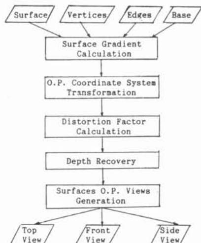
Figure 4. O.P. Views Generation Flow Diagram.
