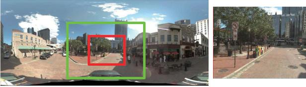
Figure 3. Features located outside the green rectangle on the panorama (left) are not used in the matching process. The red rectangle is the region that matched the previous camera frame (right)
