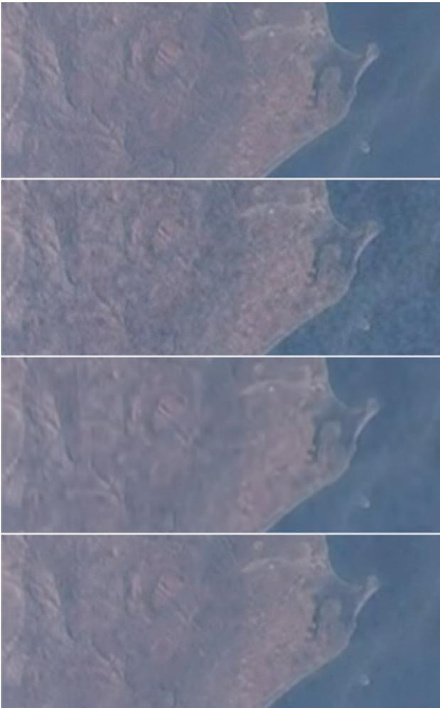
Figure 1. From top to bottom: A region of the original image, the region with noise added (coarse noise, medium magnitude), result of CVBM3D algorithm, result of the proposed HWTF algorithm.
