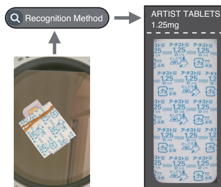
Figure 2. We propose a high-accuracy, high-speed method for recognizing blister packs. The image to the left is a query image, which was captured by our prototype. The image to the right is a reference image, which is in the image database.
