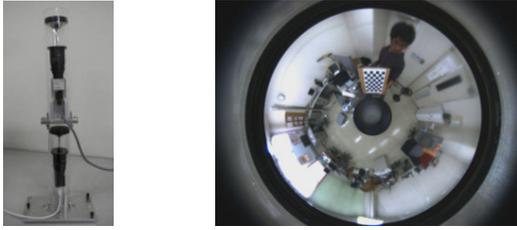
Figure 1. Onnidirectional stereo camera(left), and its image(right).
