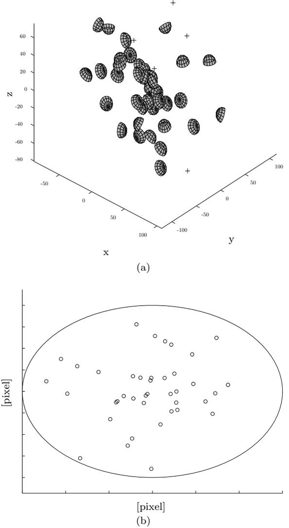
Figure 1. Synthetic data: (a) scene points (“+” marks) and fisheye cameras for 10 of the 500 vision systems; (b) image projections of such scene points (“o” marks) and boundary of the visible region (solid line).
