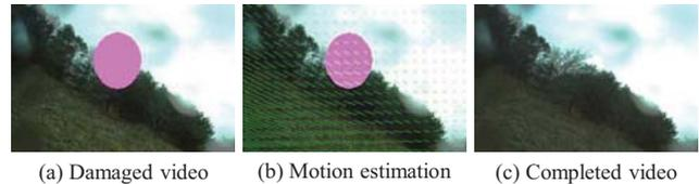
Figure 1. Video completion using the proposed method. (a) Input video with large and consecutive damage. (b) Motion estimation using the proposed method. (c) Video completion using the motion.
