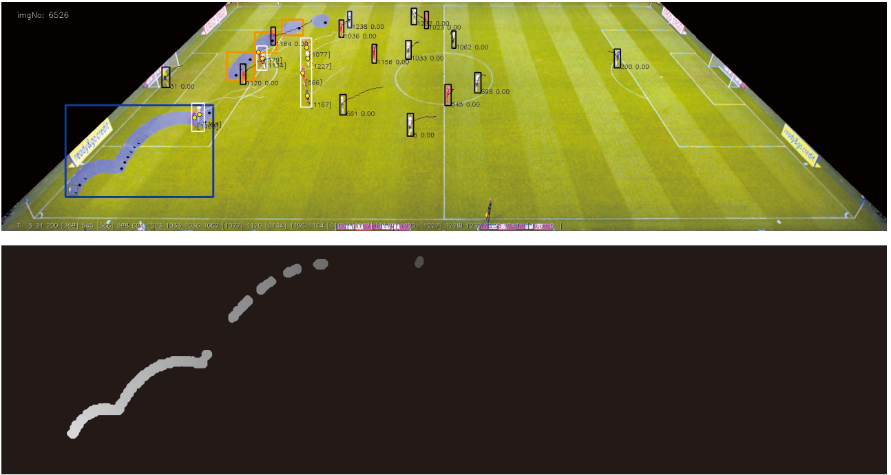
Figure 2. Sample snapshot of the processed input image sequence including detected ball tracklets (top) and one for the according motion history image (bottom).
