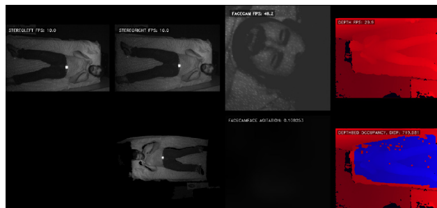
Figure 5. We can simultaneously visualize images from the all sensors alongside debugging information. Note the accurate detection of the bed in the depth field (blue mask).
