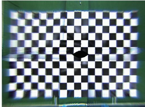
Figure 6: Integrated overhead view image
