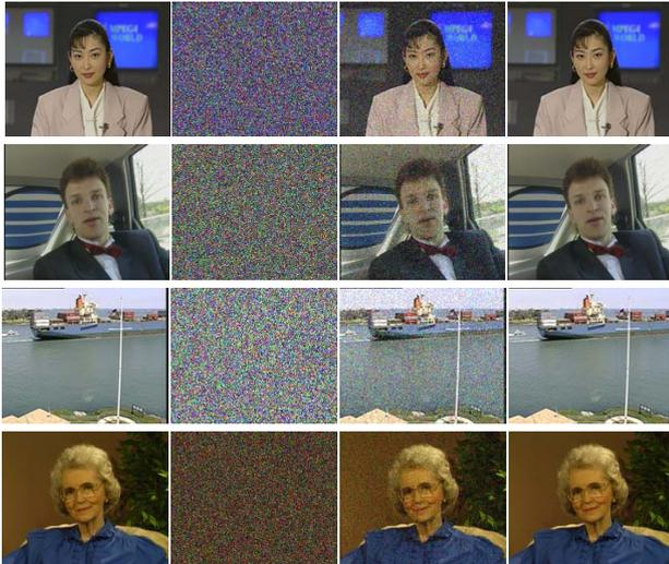
Figure 5. Sample original (the 1<sup>st</sup> column), encrypted (the 2<sup>nd</sup> column), and decrypted (the 3<sup>rd</sup> and 4<sup>th</sup> columns are using conventional [7] and adaptive methods, respectively) video frames ( $QL=8$ ; hidden data=19200 bits/frame).
