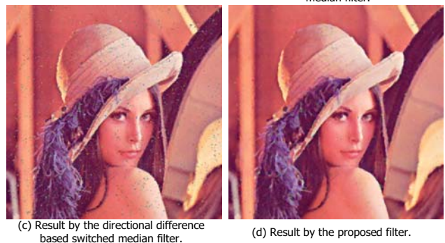
Figure 8. Comparison of different filters for the restoration of corrupted image “Lena” under the 50% impulse noise ratio.
