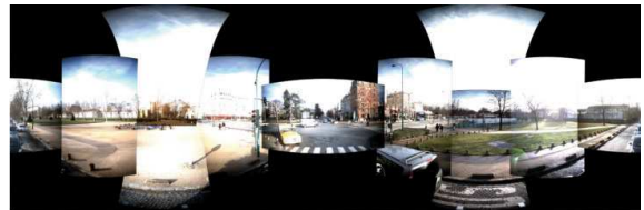
Figure 1: Example of a panoramic montage made with 10 cameras before post-processing
