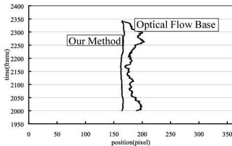
Figure 7: Lateral position of FOE on a snow road.
