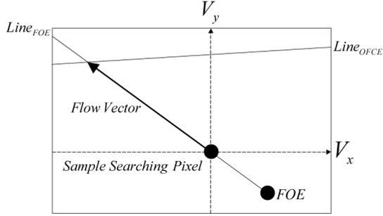
Figure 1. The intersection of  $Line_{OFCE}$  and  $Line_{FOE}$  provides the flow vector of *Sample Searching Pixel*,  $SSP_i$ .  $Line_{OFCE}$  is the line expressed by  $I_x V_x + I_y V_y + I_t = 0$
