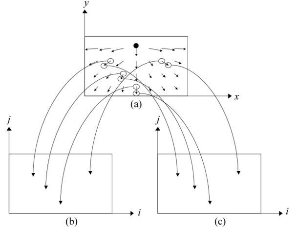
Figure 2. (a) Flow vector in the input image. (b) Warped image  $F$ , signifies the expected next frame. Each pixel is copy of  $SSP_i$ . (c) Warped image  $G$  signifies the real next frame.
