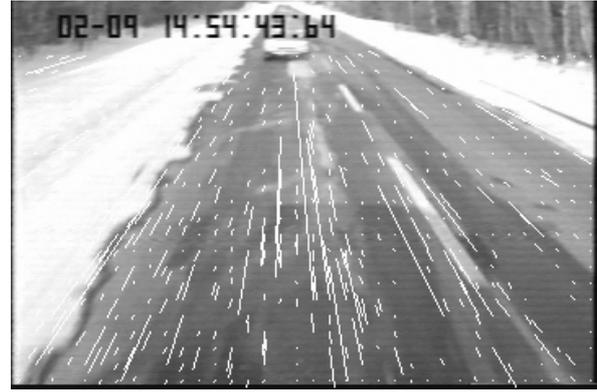
Figure 8: Vehicle on a snow road. The small lines drawn in the image show the optical flow vector, which are computed by using the position of FOE obtained from our method. The result of the optical flow shows a reasonable movement of the camera.
