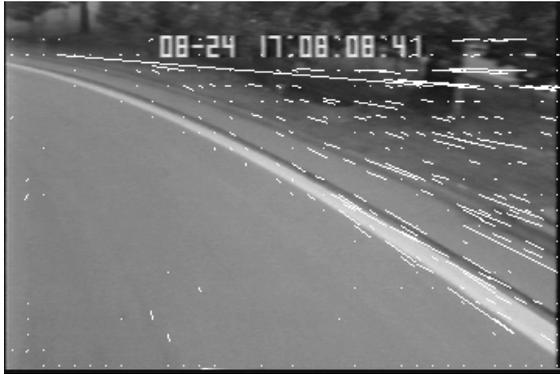
Figure 6: Vehicle on a curve. The small lines drawn in the image show the optical flow vector, which are computed by using the position of FOE obtained from our method. The result of the optical flow shows a reasonable movement of the camera.
