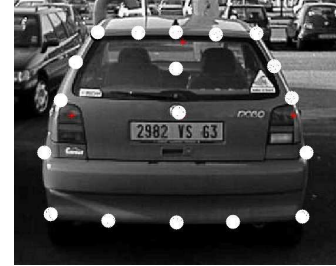
Figure 2: 18 features \mathcal{F}_i 's conforming the vehicle's model
