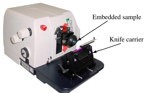
Figure 1. Microtome for cutting embedded paper samples.
