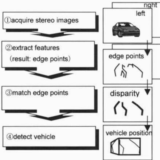
Figure 2. Vehicle position estimation using stereoscopic distance measurement
