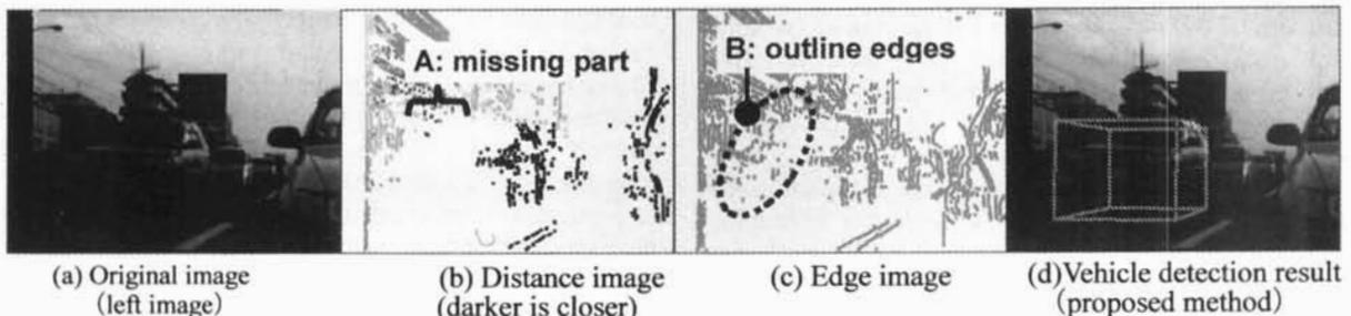
Figure 3. Result of vehicle position measurement for low light conditions in the evening
