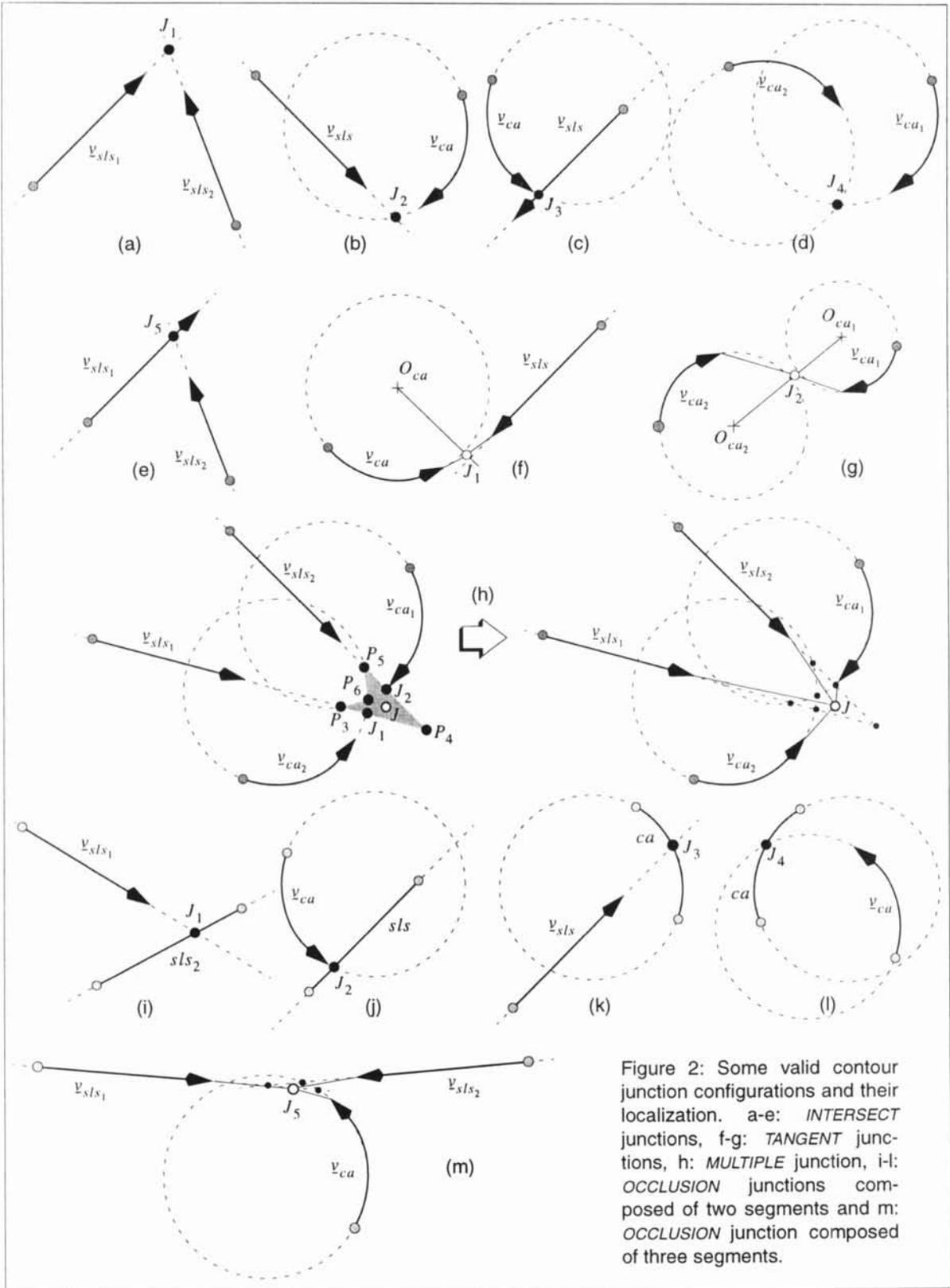
Figure 2: Some valid contour junction configurations and their localization. a-e: *INTERSECT* junctions, f-g: *TANGENT* junctions, h: *MULTIPLE* junction, i-l: *OCCCLUSION* junctions composed of two segments and m: *OCCCLUSION* junction composed of three segments.
